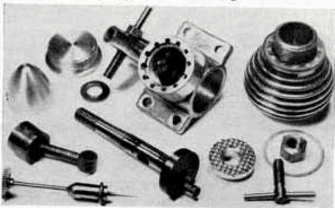
Parts of the Cormoran, showing the drilled multiple transfer passages in the main casting.
