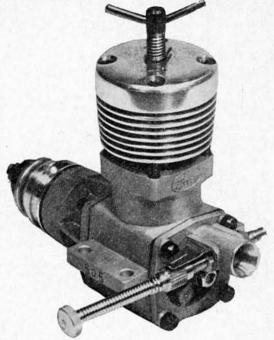
jacket held down with four bolts. The front cover carries the two ball races and crankshaft. The rear cover carrying the rotary disc valve and venturi. Both covers sealing on paper gaskets.
