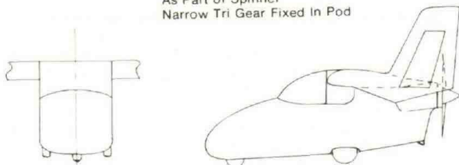
WPB-1 Mod With Simpler Pod Canted Thrust Line Tri Gear, Either Fixed Spring Type With Clean Fairing or Retractable Mains, Nose Wheel Fixed With Trouser Fairing Engine?
