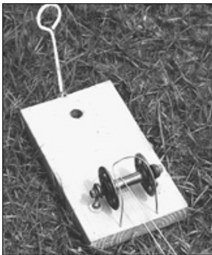
Stake is through eye screw at end of turnaround. A piece of wood this size permits the turnaround to swivel slightly on the field and align to the winch line.
