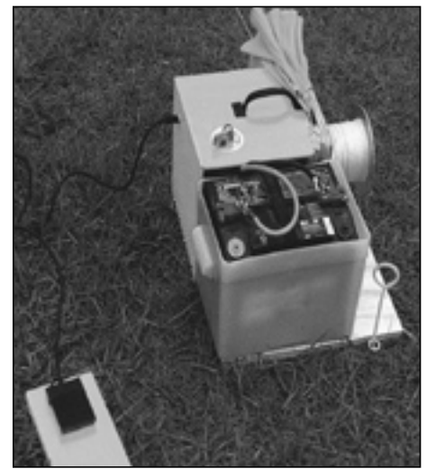
Ready for operation. Single stake aligned with line tension on reel is usually sufficient. Weight of battery on winch door makes a heavy footprint. Master disconnect switch is obvious and accessible.
